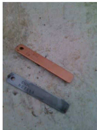
Corrosion Coupons 2 Months
